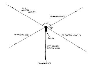
fig. 4. The parallel antenna is formed by two stagger-tuned dipoles, mounted at right angles to each other and fed at a common feedpoint.
